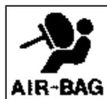
The light appears or flashes when there is a fault in the air bag system.
