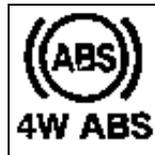
The light appears when there is a fault in the Antilock Braking System.
