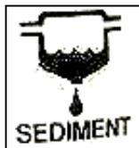
The light appears when the water level in the fuel sedimentation tank exceeds the limit.
