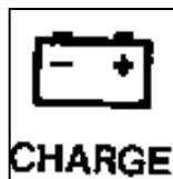
The light appears when there is a fault in the battery charging system.
