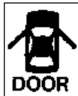
The light appears when any of the doors are not properly closed.
