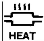
The light appears when the temperature of the catalytic converter is abnormally high.
