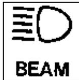
The light appears when the headlights are on high/main beam.
