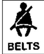
The light appears when the driver's seat belt is not fastened.
